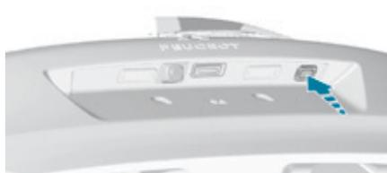
Locking is confirmed by fixed illumination of the direction indicators for a few seconds. Depending on version, the door mirrors fold and the alarm is activated.
