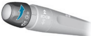
**O** Lighting off (ignition off) / Front daytime running lamps (engine running).
