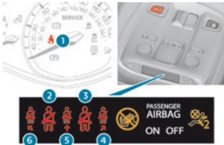
1. Front and/or rear seat belts not fastened / unfastened warning lamp in the instrument panel.
