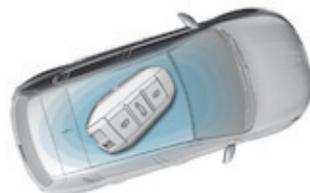
With the Keyless Entry and Starting remote control inside the vehicle, pressing the "START/STOP" button, **with no action on the pedals**, allows the ignition to be switched on. This also allows the accessories to be used (for example: audio system, lighting...).
