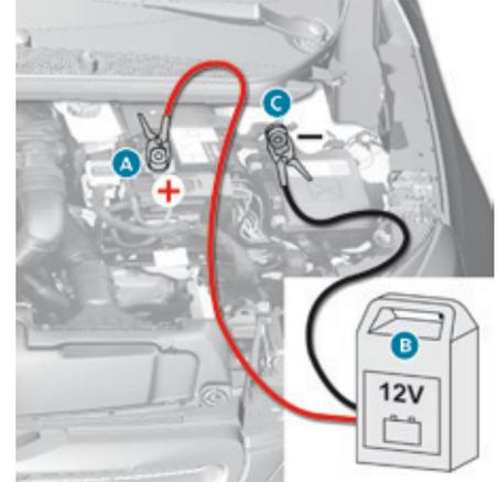
**!** Never try to charge a frozen battery. If the battery has been frozen, have it checked by a PEUGEOT dealer or a qualified workshop, who will check that the internal components have not been damaged and the casing is not cracked, which could cause a leak of toxic and corrosive acid.
