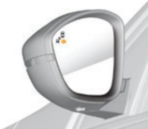
Each fitted with an adjustable mirror glass providing the lateral rearward vision necessary for overtaking or parking. They can also be folded for parking in confined spaces.
