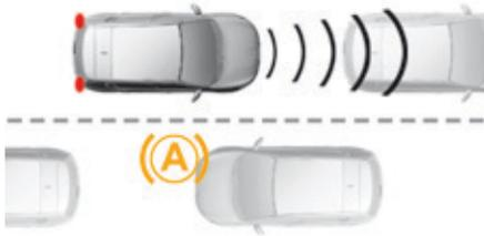
Emergency collision braking is a system that aims to reduce the speed of a frontal collision if the driver does not take action, using radar type detection and acting on the vehicle's braking system.
