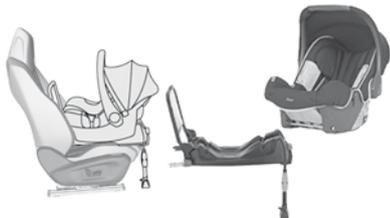
Installed rearward facing using an ISOFIX base which is attached to the rings **A**. The base has a support leg, adjustable for height, which sits on the vehicle's floor. This child seat can also be secured with a seat belt. In this case, only the shell is used and attached to the vehicle's seat by the three-point seat belt.
