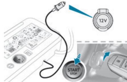
☞ Connect the compressor's electric plug to the vehicle's 12 V socket.
