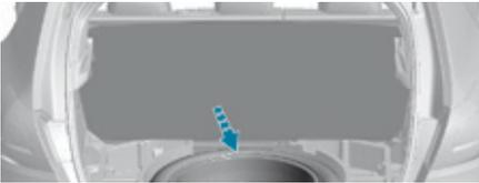
The spare wheel is located in the boot under the floor.
