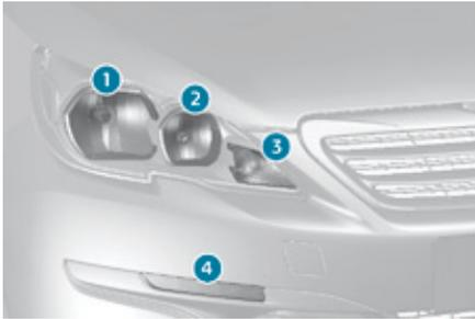
1. Dipped beam headlamps (H7-55W).
