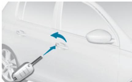
Turn the key towards the rear of the vehicle to fully lock the vehicle.
