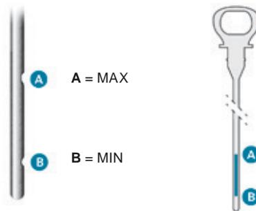
If you find that the level is above the **A** mark or below the **B** mark, **do not start the engine**.
