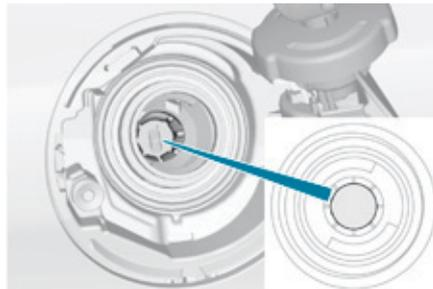
**i** It is still possible to use a fuel can to fill the tank but this must be done slowly. In order to ensure a good flow of fuel, do not place the nozzle of the fuel can in direct contact with the flap of the misfuel prevention device.
