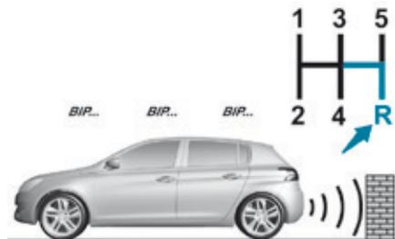
The proximity information is given by an intermittent audible signal, the frequency of which increases as the vehicle approaches the obstacle. The sound emitted by the speaker (right-hand or left-hand) indicates the side on which the obstacle is located.
