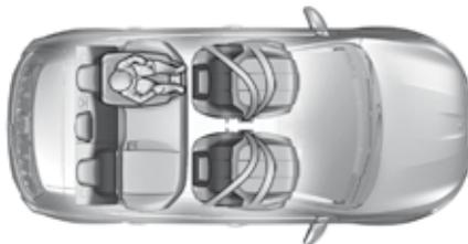
When a forward facing child seat is installed **on a rear passenger seat**, move the vehicle's front seat forward and straighten the backrest so that the legs of the child in the forward facing child seat do not touch the vehicle's front seat.
