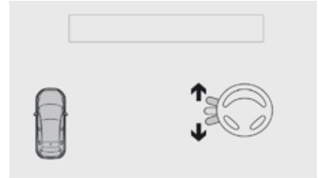
☞ Operate the direction indicator on the parking side chosen to activate the measurement function. You should drive at a distance of between 0.5 m and 1.5 m from the row of parked vehicles.
