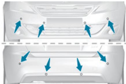
This system indicates the proximity of an obstacle (e.g. pedestrian, vehicle, tree, gate) which comes within the field of detection of sensors located in the bumper. Certain types of obstacle (e.g. stake, roadworks cone) detected initially will no longer be detected at the end of the manoeuvre, if they are located in blind spots in the sensors' field of detection.
