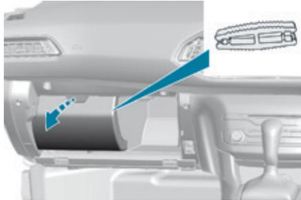
The extraction tweezer is fitted to the back of the dashboard fusebox cover.
