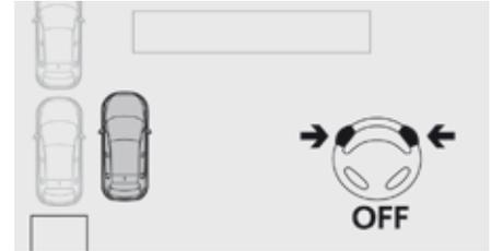
The manoeuvre is complete when the vehicle's front wheels are clear of the parking space. At the end of the manoeuvre, the indicator lamp in the instrument panel goes off, accompanied by a message and an audible signal. The assistance is deactivated: you can take over control.
