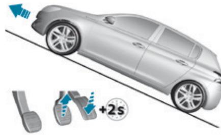
**On an ascending slope, with the vehicle stationary, the vehicle is held momentarily when you release the brake pedal.**
