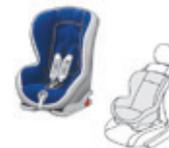
Is installed only in the forward facing position. Is attached to the rings **A** and the upper ring **B**, referred to as the TOP TETHER, using an upper strap. Three seat body angles: sitting, reclining, lying down. This child seat can also be used on seats not equipped with ISOFIX mountings. In this case, it must be secured to the vehicle's seat by the three-point seat belt. Adjust the position of the vehicle's front seat so that the child's feet are not touching the backrest.
