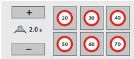
Press button **5**, the six memorised speeds and the inter-vehicle time setting are displayed in the touch screen.
