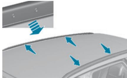
You must attach the transverse bars at the engraved markings on the longitudinal bars.
