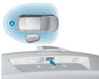
☞ With the electronic key on your person in the recognition zone **A**, press the opening control then raise the tailgate.
